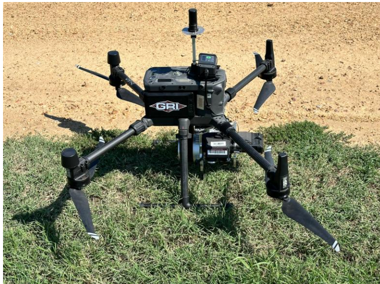
Figure 9: Geocue Trueview 515 3D Imaging System
