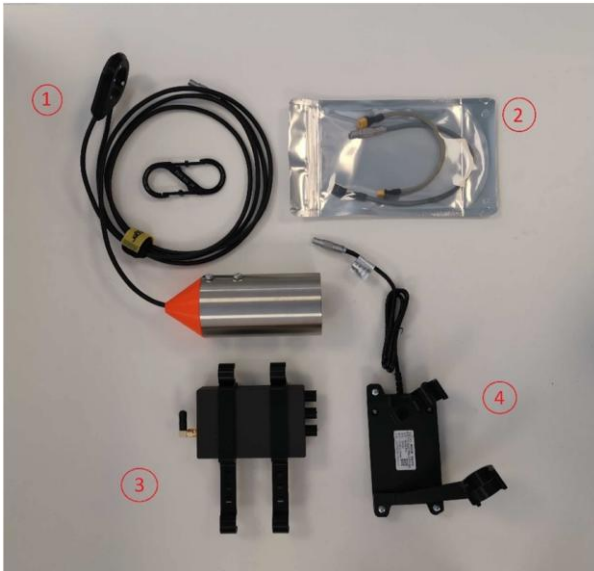
Figure 2: Echo-sounder and its mandatory hardware components
